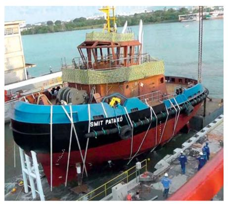
Launching of the first of six Azimuth Stern Drive (ASD) harbour tugs to be delivered to SMIT Rebras at Keppel Singmarine Brasil
