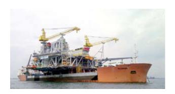
Completed by Keppel FELS in Singapore, the topside module of the P-61 Tension Leg Wellhead Platform (TLWP) has arrived in Brazil after a 17,000 km journey from Singapore. It will be joined to the lower hull which is being fabricated at Keppel FELS Brasil's BrasFELS yard in Angra dos Reis. When fully integrated, the P-61 will be the first such platform in Brazil and will be deployed to the Papa Terra field in the southern section of Campos Basin, 100 km from Cabo Frio, Rio de Janeiro.
