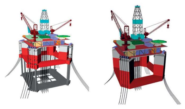
KOMtech and FloaTEC have developed the Extendable Draft Semisubmersible (left) and Deep Draft Semisubmersible (right) to provide companies with alternative dry tree solutions
