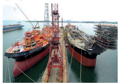
Bumi Armada's FPSO Armada Sterling (on left) and FPSO Armada Claire (on right) are seen docked side by side at Keppel Shipyard. Armada Sterling is the tenth project to be completed by Keppel Shipyard for long-term customer Bumi Armada. FPSO Armada Claire is currently undergoing refurbishment and upgrading works at the yard
